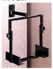
Ceiling Bracket 14" - 20" with Cradle Monitor Width: 320mm to 530mm Monitor Height: 435mm to 500mm Distance from wall to cradle centre 500mm
